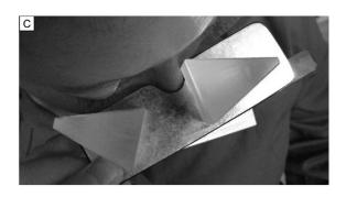
Each prism is held level by the plate avoiding induced vertical prism. When necessary, an additional prism with power up to  $20\Delta$  containing a magnet in the base can be positioned base down in front of either horizontal prism to neutralize combined horizontal and vertical deviations (see Figure D).
